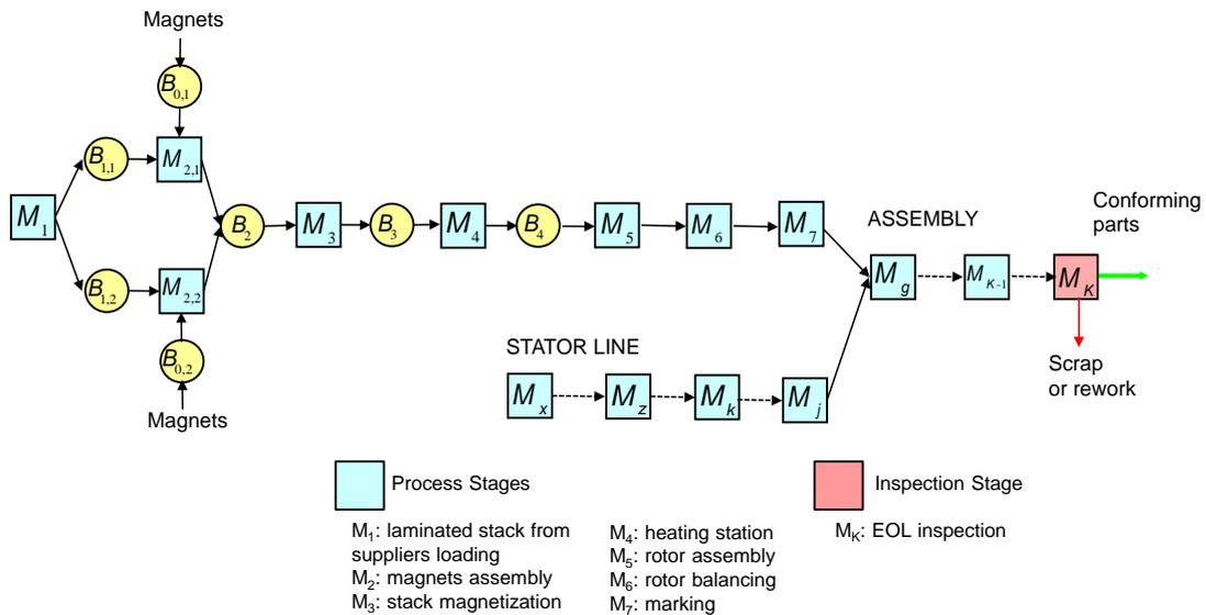
Fig. 3. Current production line for electric drives with EOL inspection.
