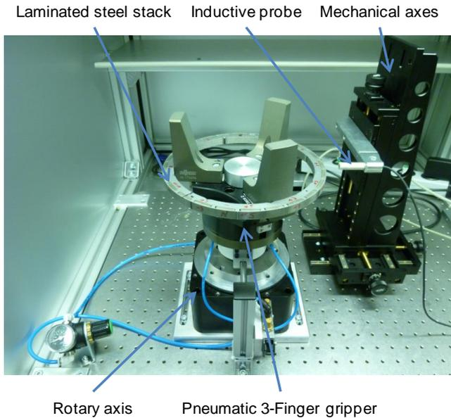
Fig. 4. Main components of the preliminary test bench for space resolved measuring of the magnetic field.
