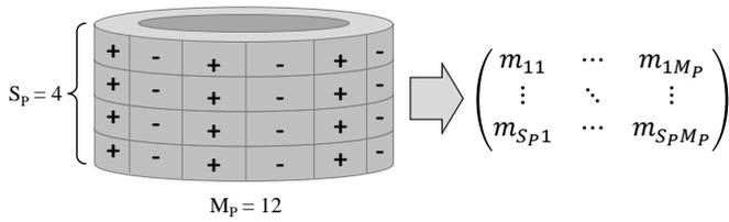
Fig. 2. Rotor consisting of  $S_P = 4$  stacks and  $M_P = 12$  magnets (matrix dimensions  $4 \times 12$ ).
