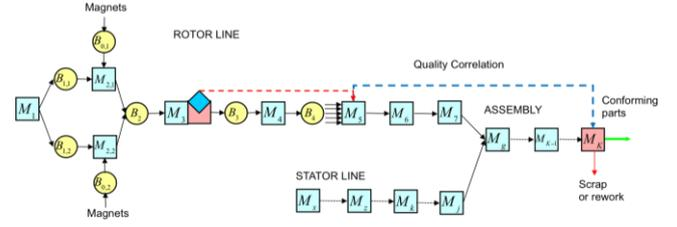
Fig. 7. Reconfigured line including on-line inspection and new sequential proactive assembly strategy.
