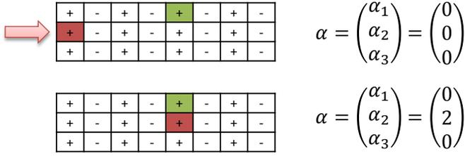
Fig. 6. Stack number two is shifted to the right in order to compensate the weak magnet at position one by the stronger magnet at position 5 of the first stack.
