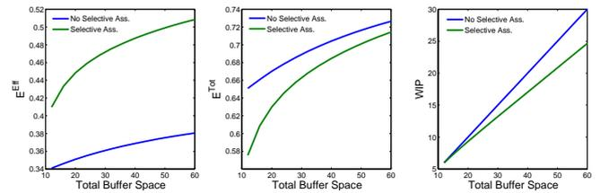
Fig. 9. Impact of the selective assembly strategy on the system performance.  $E^{\text{Tot}}$  is the total throughput of both conforming and non-conforming assemblies,  $E^{\text{Eff}}$  is the effective throughput of only conforming assemblies, WIP is the work in progress.
