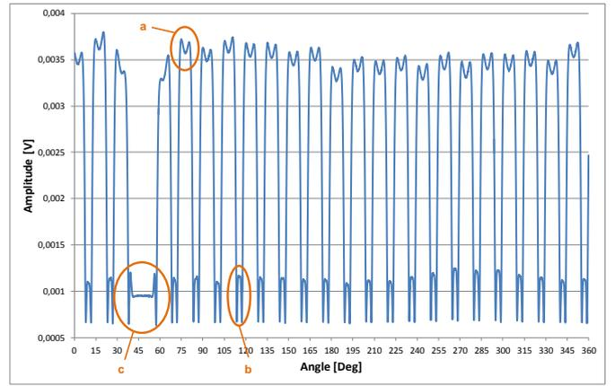
Fig. 5. Space resolved measurement of the magnetic field of a laminated steel stack with an artificial defect (here sensor output in V).
