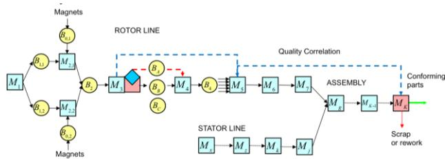
Fig. 8. Reconfigured line including on-line inspection and new selective assembly strategy.
